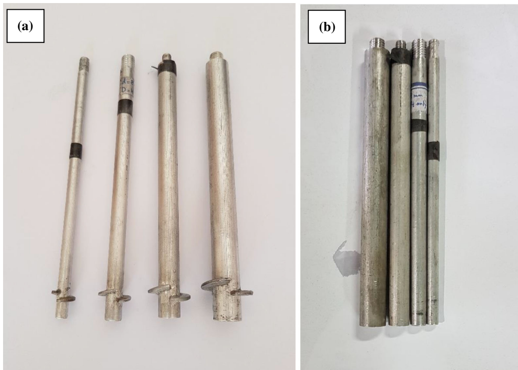
Fig. 5 Physical models of (a): helical anchors and (b): shaft-only
